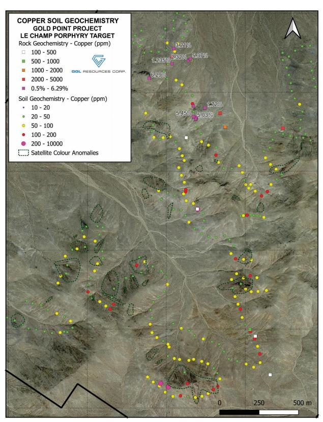
Interpretation of satellite imagery has identified numerous limonite-stained talus trains within the intrusion that are believed to represent leached areas within the upper portions of a buried porphyry system. Areas
